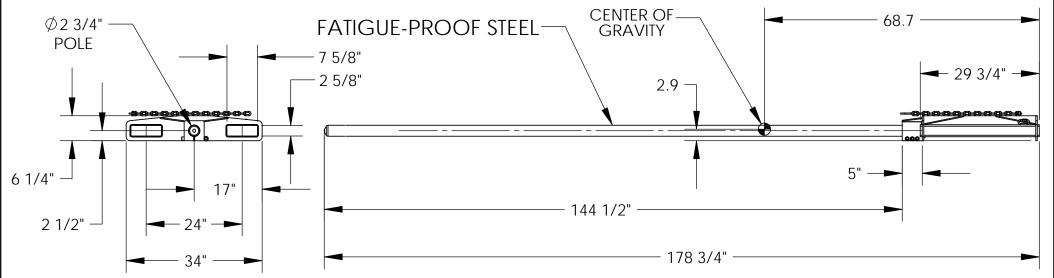
HORIZONTAL CENTER OF GRAVITY: 68.7" VERTICAL CENTER OF GRAVITY: 2.9 LOST LOAD:420 LBS. (APPROX.)
