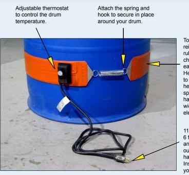
Tough fiberglass reinforced silicone rubber band is flexible, chemical resistant, and easy to keep clean. Heater band conforms to the drum surface, held in contact by spring tension. Heaters have a 4" (10.16 cm) wide with heating elements.
