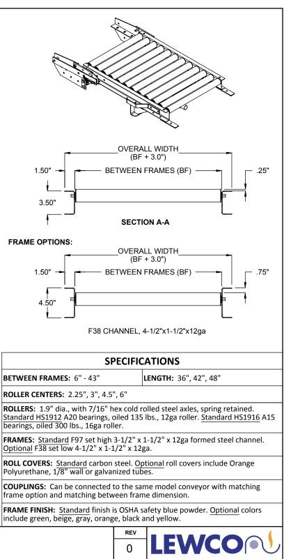
Model: HS1912, HS1916 - Spring Assisted Hinge Gate, 1.9 diameter roller
